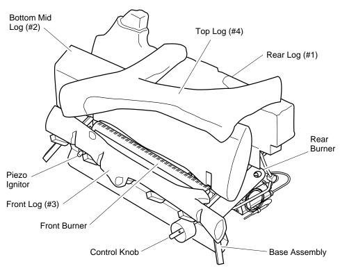
Figure 1 - Vent-Free Gas Log Heater
